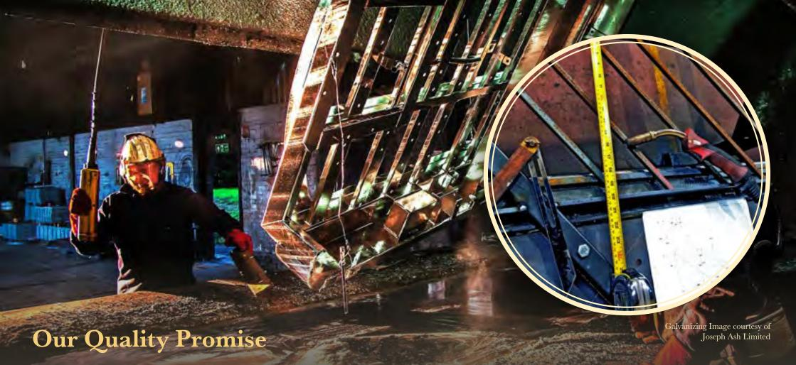
At Heartlands Metal Craft, our manufactured gates go through a Hot Dip Galvanizing process\* to prevent the steel from corroding, giving customers peace of mind that their metal craft will have a long life and be easy to maintain.
